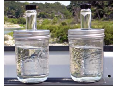
The effluent sample on the left, discharged from an Orenco AX100 Treatment System, is as clear as the water sample on the right, taken from a nearby lake.
