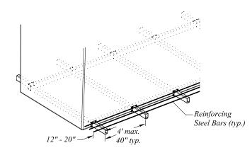
Anti-Flotation Framework Detail
