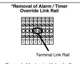
Removal of the terminal link rail will separate the high level alarm and override timer functions.
