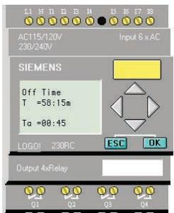
Step 6: When the desired time value has been entered, press the “OK” key. The new time value will now be in effect.
