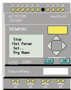
Step 2: Press **▼** on the unit to select “Set Param.” Then press the “OK” key.
