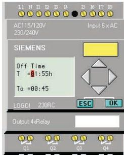
Step 4: The first line indicates the set value for the parameter. In this example, the set time is 1 hour and 55 minutes, “T=01:55h.” To change the set value for the parameter, press the “OK” key.
