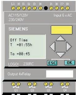
Step 3: Press  $\blacktriangle$  or  $\blacktriangledown$  to view the parameter values. In this example, “Off Time” is being viewed.
