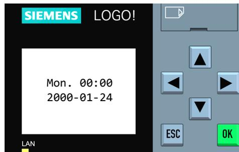
**Step 8:** To go back to the list of all adjustable parameters press the “ESC” key once and return to **Step 4**. When all edits are complete, exit parameter mode by pressing the “ESC” key four times.
