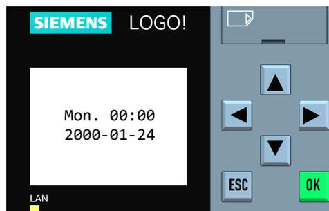
**Step 8:** To edit additional parameters, go back to the parameter list by pressing the “**ESC**” key once and return to **Step 4**. When all edits are complete, exit parameter mode by pressing the “**ESC**” key four times.
