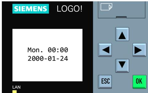
**Step 1:** Press  $\blacktriangledown$  repeatedly until the display does not change. To begin the configuration process, press the "ESC" key.
