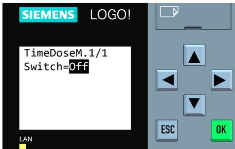
**Step 7:** When the desired value has been entered, press the "OK" key. The new value will now be in effect.
