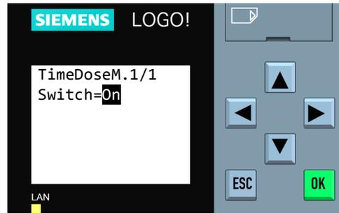
**Step 6:** The cursor will blink on the switch parameter. To change the value of the softkey switch, press ▲ or ▼. In this example, the set value has been changed from "On" to "Off".
