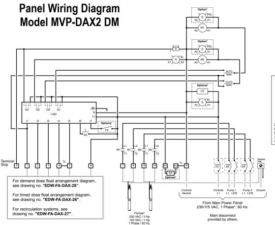
NOTE: Motors must have internal overload protection
