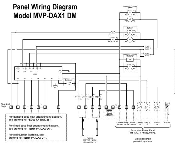
NOTE: Motors must have internal overload protection
