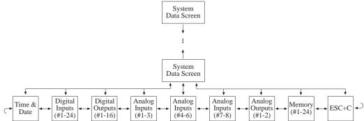
**Input and Output Screens:** The unit will activate various inputs and outputs as it operates (please refer to the Liquid Crystal Display screens shown below). Knowing what conditions cause the inputs and outputs to activate can be a helpful installation and troubleshooting tool. The following inputs and outputs have been used with your control panel:
