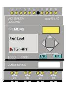
Step 5: The cursor will appear on the switch parameter. To change the value of the softkey switch, press ▲ or ▼. In this example, the set value has been changed from "Off" to "On."
