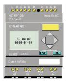
Step 7: To exit parameter mode, press the "ESC" key twice.
