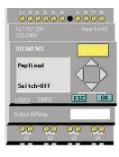
Step 4: The bottom line indicates the current state of the softkey switch. In this example, the softkey is set to "Off." To change the set value for the parameter, press the "OK" key.
