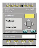
Step 3: Press ▲ or ▼ to view the parameter values. In this example, "**Pmp1Lead**" is being viewed.
