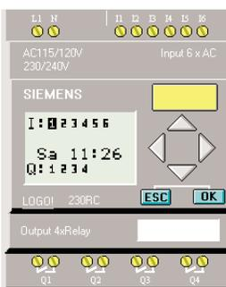
Step 7: To exit parameter mode, press the "ESC" key twice.
