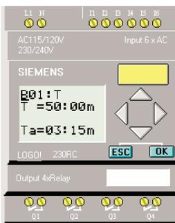
Step 6: When the desired time value has been entered, press the "OK" key. The new time value will now be in effect. To set additional parameters, repeat Steps 3-6.
