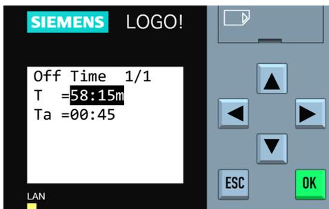
**Step 7:** When the desired time value has been entered, press the “OK” key. The new time value will now be in effect.
