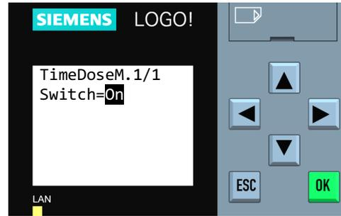
**Step 6:** The cursor will blink on the switch parameter. To change the value of the softkey switch, press  $\blacktriangle$  or  $\blacktriangledown$ . In this example, the set value has been changed from "On" to "Off".
