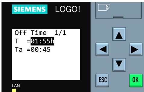
**Step 5:** The first line indicates the set value for the parameter. In this example, the set time is 1 hour and 55 minutes, “T=01:55h.” To change the set value for the parameter, press the “OK” key.
