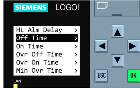
**Step 4:** Press  $\uparrow$  or  $\downarrow$  to select the desired parameter to adjust and press “OK”. Continue to **Step 5** on the following pages for the specific block type being edited.
