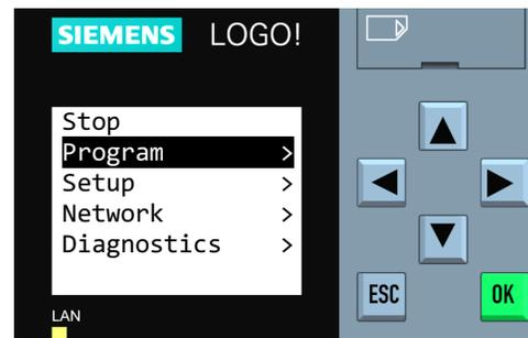
**Step 2:** Press ▼ on the unit to select "Program". Then press the "OK" key.
