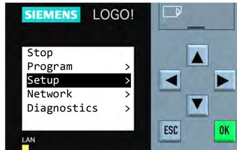
Step 1: Press ▼ repeatedly until the display does not change. To begin the configuration process, press the "ESC" key.
