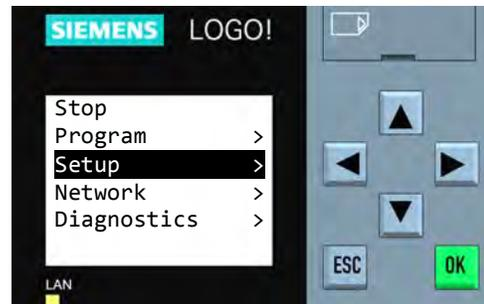
Step 2: Press ▼ twice to select “Setup”. Then press the “OK” key.
