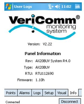
The “Rev” displays the program name, and revision number of the program running in the VeriComm board.
