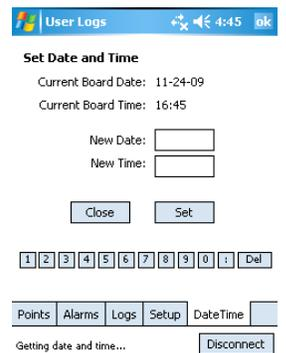
The current date and time on the VeriComm board will appear after a few seconds as the BT-VCOM program retrieves the data. You may enter a new date and time by clicking in the “New Date” and “New Time” text entry boxes and then using the numeric keypad below to enter the values.
