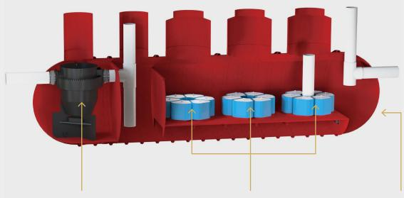
The **Prime Separator** removes trash and debris, and petroleum hydrocarbons, suspended solids and heavy metals. Filter Cartridges remove liquidbound and sediment-bound nutrients and metals, hydrocarbons, heavy metals and solids The watertight, corrosionresistant **HydroChain Tank** is available in diameters of 8' to 15.5'
