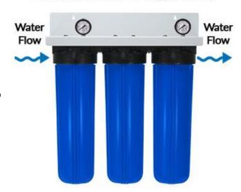
Includes (2) 2" pressure gauges installed to easily and quickly show you when it is time to change your filters. A decrease in water flow of 7 PSI differential indicates the filter cartridge should be replaced.
