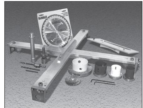
For cutting Perma-Loc, Ultra-Rib, KOR FLO, and Ultra-Corr pipe in the field and preparing pipe for grommets/lid attachment.
