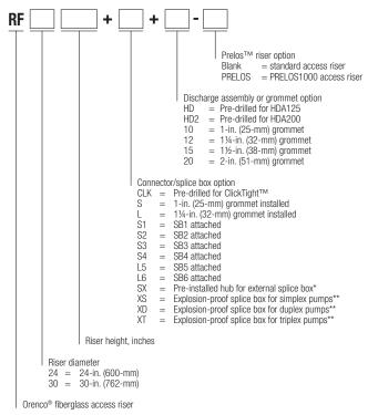
\* Minimum riser height 18-in. (457-mm) \*\* Used in Class I Division 1 environments
