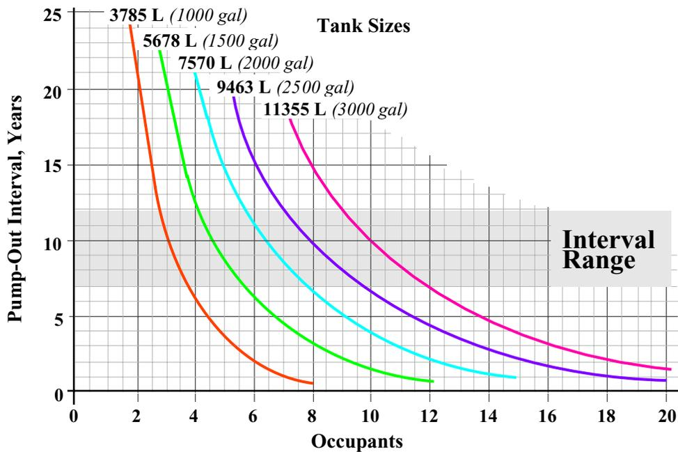
Figure 4: Pump-Out Intervals at 95% level of Confidence
