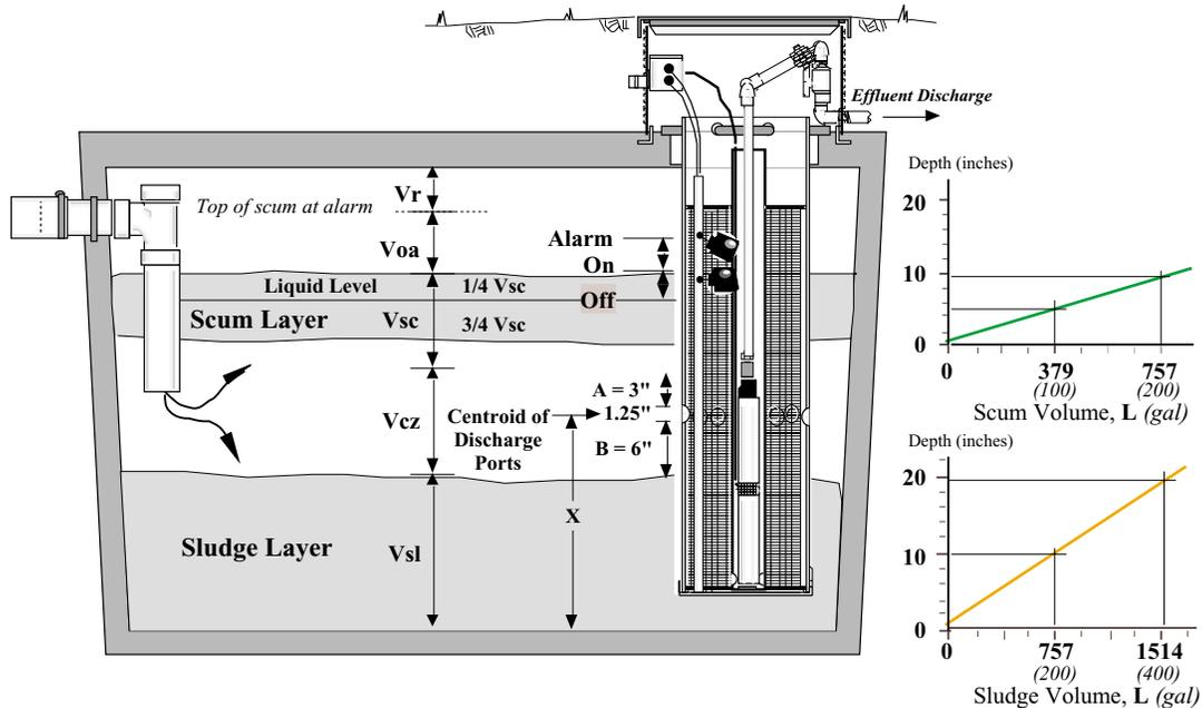
Figure 2: Typical 3785 L (1000 gal) concrete dosing septic tank
