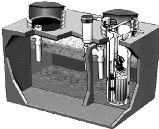
**Figure 8: Typical Dosing Septic Tank
