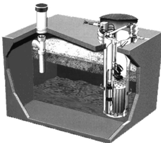
Figure 6: Typical Dosing Septic Tank
