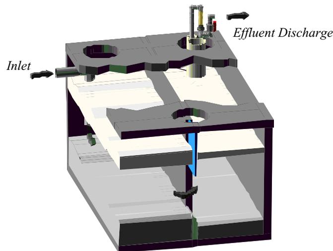
**Figure 9: Partition Tank Configuration with Removable Scum Baffle**
