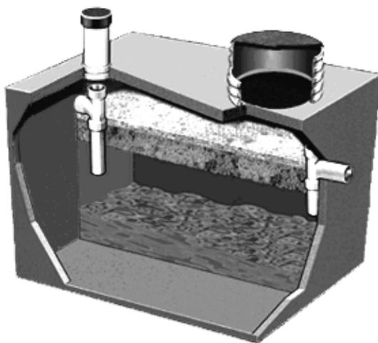
Figure 5: Typical Gravity Septic Tank
