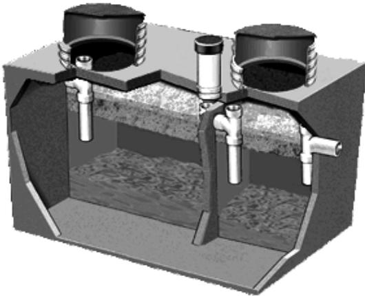
**Figure 7: Typical Gravity Septic Tank
